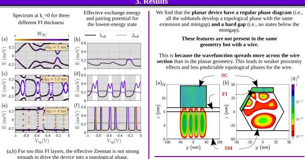
**Conclusion.** – This planar platform support predictable and robust topological states. Since they are based on 2DEG, they present reduced disorder in comparison to a wire. And because there is no need of a magnetic field, different effective wires could have different orientations. Hence, this geometry is promising for QC.
